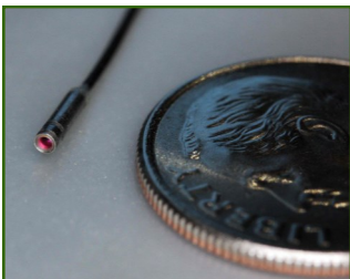
The main feature of VIPIR is a tiny micro camera that is only about 1mm in diameter, thinner than a dime. Contained in this small space is the optics, the imager and the electronics needed to send the image electronically to the VPU (right).
