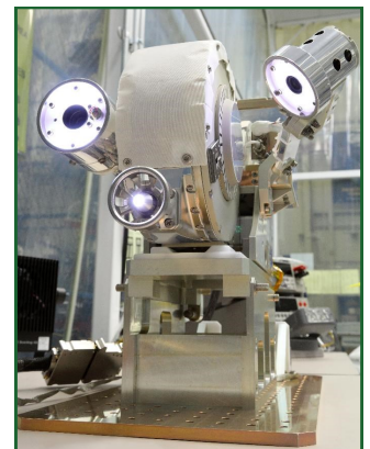
The assembled VIPIR. The micro camera is the bottom most camera, and has a ring of white LEDs surrounding it.
